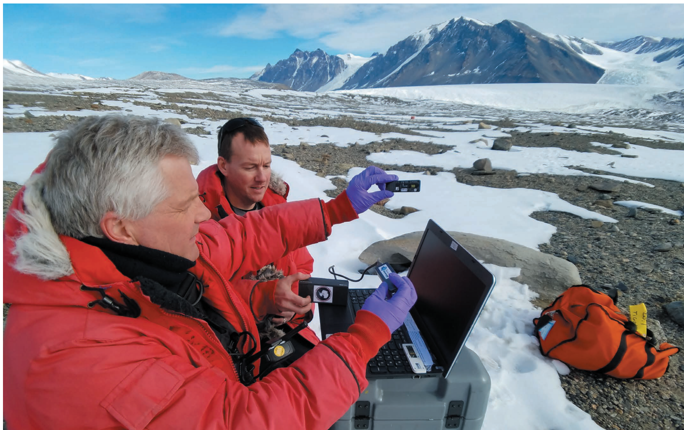
Scott Tigue (left) and David Goerlitz use the MinION device to sequence microbial DNA in Taylor Valley, Antarctica.
