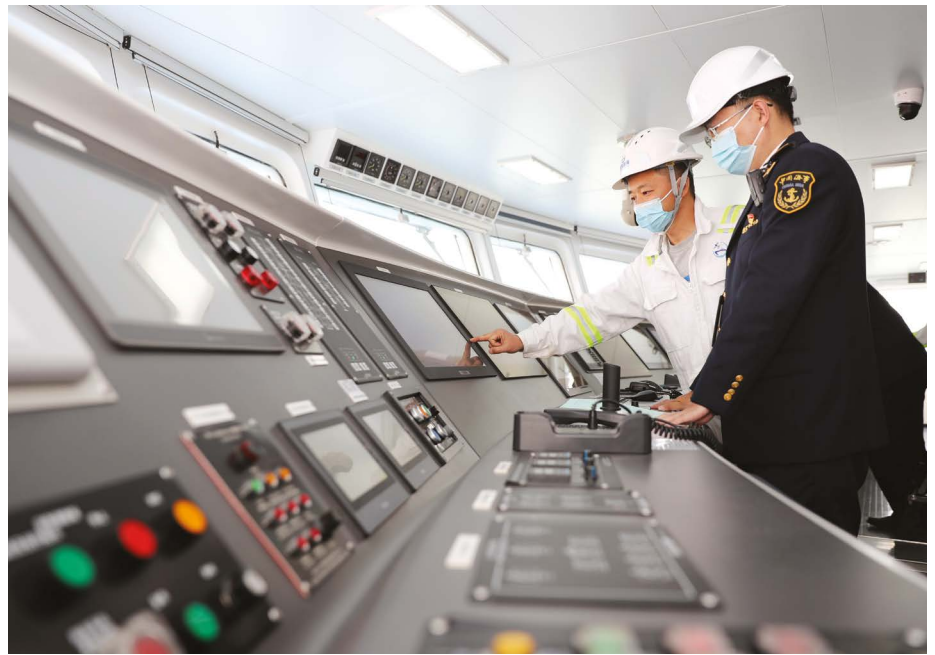
Interactions between humans and autonomous ships will need to be redefined, as for the Chinese ship Zhi Fei, which operates under remote control.
