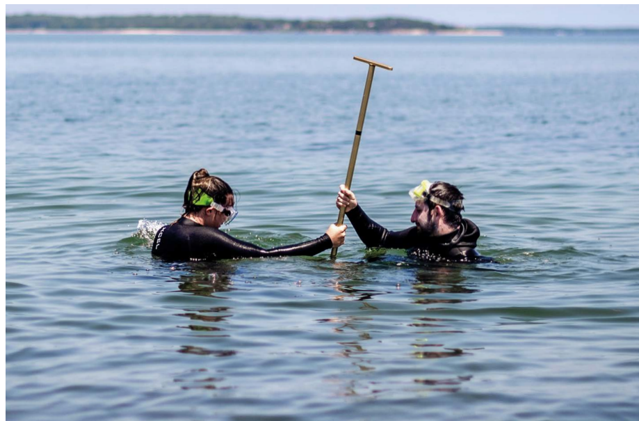
A team takes a core sample of ocean bottom sediments at North Sea Beach, New York.
