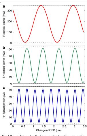
Fig. 3 Dependence of optical power after interference on the change in OPD. a Fundamental light; b SH light; c FH light
