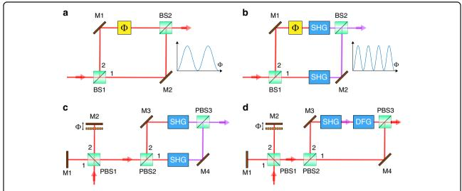
Fig. 1 Schematics of the interferometer configurations. a MZI. b Nonlinear MZI. c Nonlinear polarized interferometer. d Configuration for phase doubling without frequency doubling
