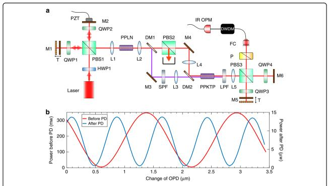
**Fig. 4 Experimental setup and results. a** Experimental setup used for phase doubling (PD) without frequency doubling. SPF: 1000 nm short pass filter; LPF: 1400 nm long pass filter; FC: fibre collimator; CH22: channel 22 of a dense wavelength division multiplexing system with a centre wavelength of 1559.79 nm. **b** Measured optical power characteristics of interference before and after phase doubling
