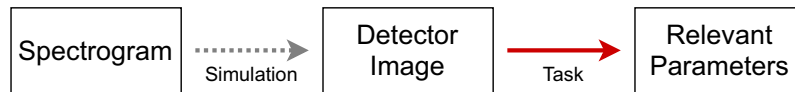
Figure 7. We use a simulated spectrogram to construct according detector images. These images are used for training the NNs and to extract several different pulse characteristics afterward.
