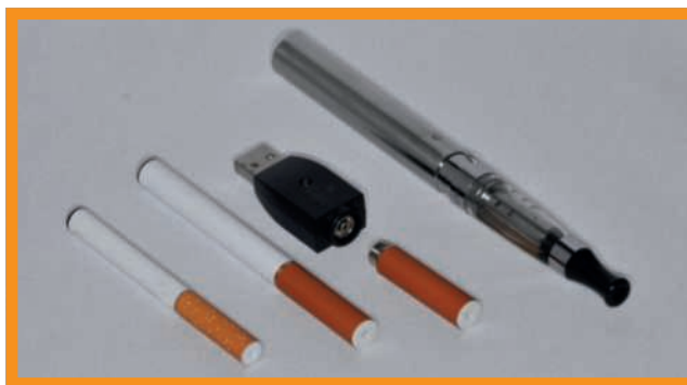
Fig. 1 Three types of e-cigarettes: disposable e-cigarette; rechargeable cartridge e-cigarette; and rechargeable liquid refillable e-cigarette, photographed by PSP Worsley
