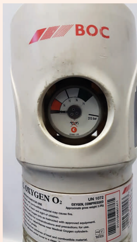
Fig. 2 Oxygen cylinder needs replacing as it is in the 'red zone'
