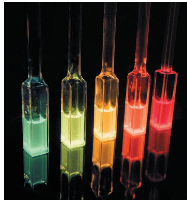
▲ A new type of quantum dot has the benefit of being free from some of the common toxic materials found in conventional quantum dots. Quantum dots are fabricated by a commercial-scale manufacturing process to reliably produce particles with a specific peak luminescence wavelength.
